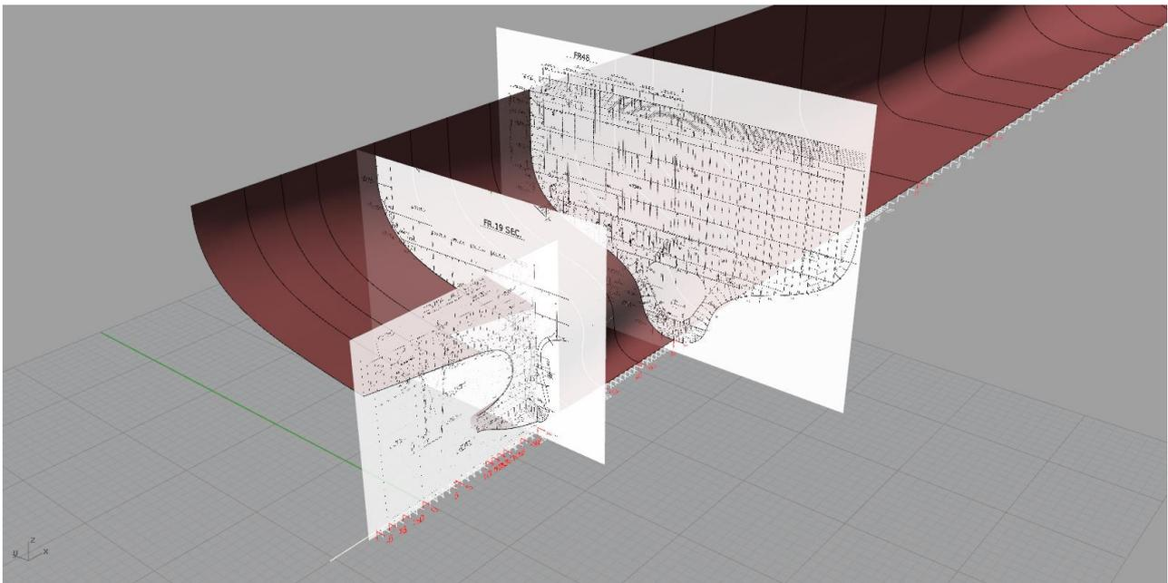
Figure 4: Example of a frame based 3D hull surface showing selected underlying frames and pictures
